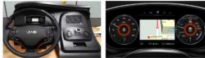
Fig. 18. Automotive digital cluster hardware and display.
